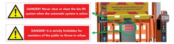
The additional safety decals shall be offered on a free of charge basis to all customers with existing products in service.
