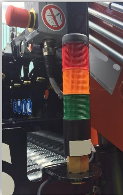
Figure 2: A typical RCI / RCL visual warning device
