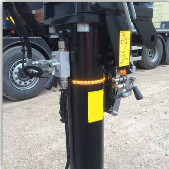
Figure 3: Use of stabiliser leg lights as Operational warnings
