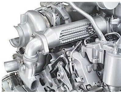
Figure 8: An example of a tubular EGR cooler 11
