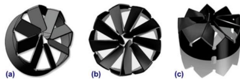
Figure 12: Examples of DEF mixers for light-duty applications 14
